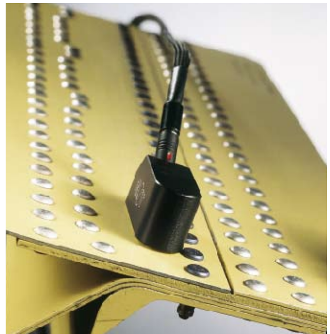
MDK-1 probe for checking for cracks in the riveted plate
